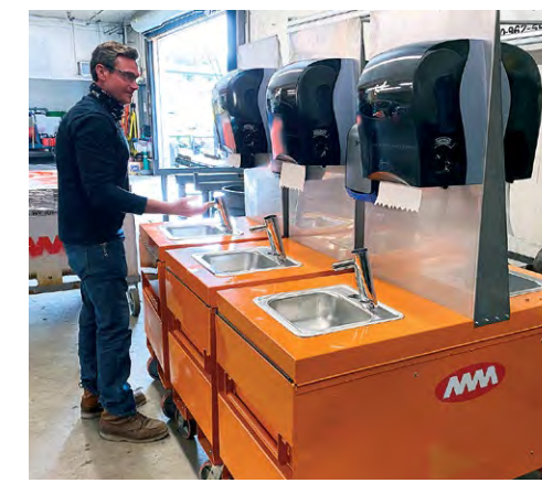
Another round of portable hand washing stations complete with touchless dispensers. Shout out to Plumbing Shop Foreman, Justin Guy for quality checking the dispensers before shipping!
